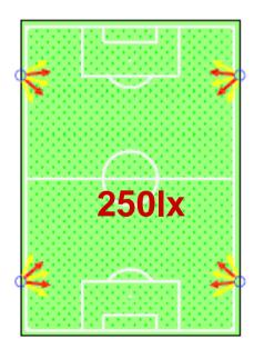
250 lx = 4 poles with light point heights of 18m 20 pcs. LED headlights and electrical components
